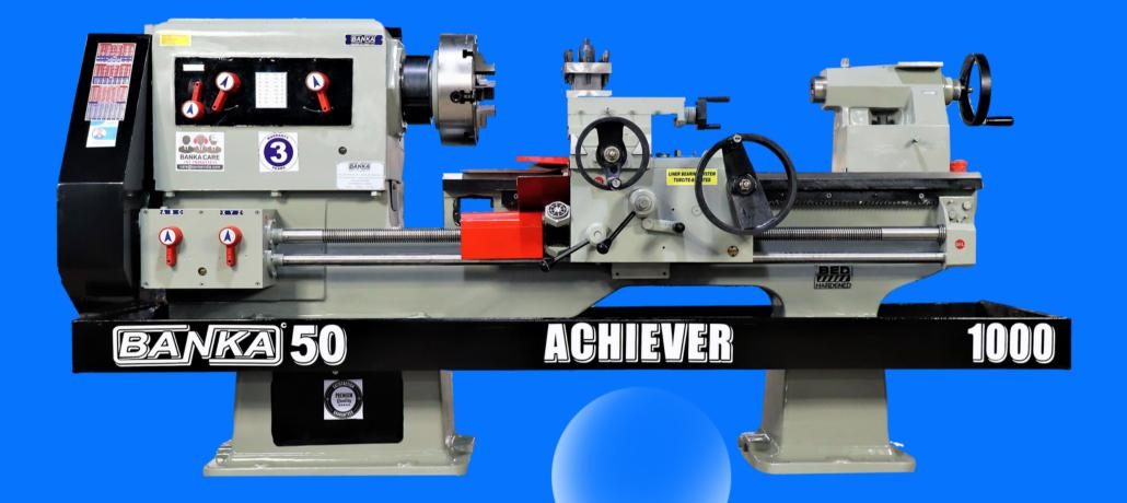
Height Of Center: 250 mm Spindle Bore: 80 mm Admin Between Center: 1000/1500/2500/3000 mm Spindle Speed: 1050 RPM Bed Width: 260 mm
